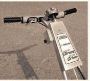
**Electric deadman switch** insures operator safety and security.
